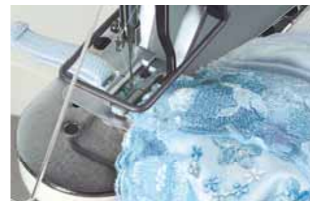
F type (Attaching the shoulder straps to brassier) *Presser foot for vertical bartacking is supplied with the unit as an accessory.
