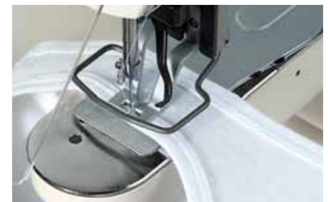
M type (Bartacking shoulder of running shirt)
